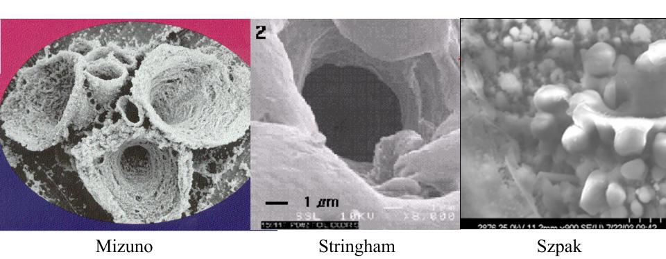
Chemical energies are insufficient to cause the craters that have been observed on cathode surfaces in many "cold fusion" experiments
