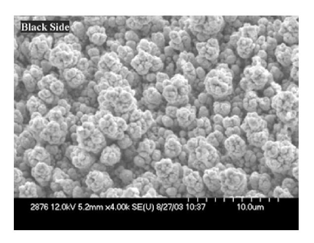
Pd/D structure before Application of external Electric field.
