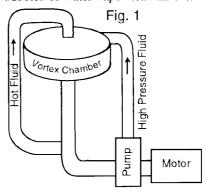
As shown in the figure, there is a secondary circulation. Because the wall pressure higher than pressure at the center o f the vortex chamber, there is a secondary flow from the down pipe back to the center of the
