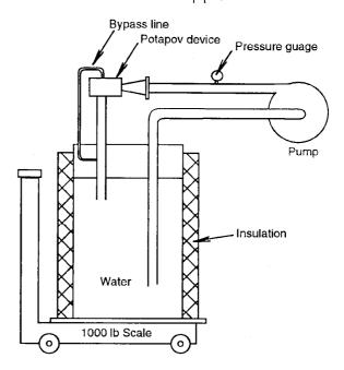
The bypass line connects the secondary outlet to the main exit pipe. This line appears to be an optional feature of the Potapov device. In the literature accompanying our YUSMAR-2, the bypass line is not shown. However, in a photograph we obtained which shows a device similar in size to the YUSMAR-2, the bypass line is clearly present. We conducted tests with and without this line.
