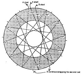
I have a good stock of #24 enamel wire so used this throughout. Each completed winding consists of a number of turns laid side-by-side around the outside each connecting segment crossing over the previous ones as it passes through the center. This is necessary to insure the outer turns progress in the same direction for each wrap, to the left or right of each preceding wrap.
