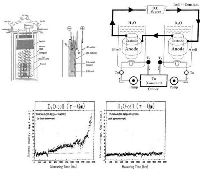
Figure 2 : The Arata Zhang double cathode experiment
