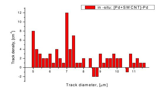
Pd/SWCNT/Pd after electrolysis: t = 10 x 3600 s, open CR-39 data:  $\langle N_p \rangle = (1.7\pm0.7)x10^{-3} \text{ p/s-cm}^2;$  $\langle N_\alpha \rangle = (2.8\pm0.9)x10^{-3} \alpha/\text{s-cm}^2$
