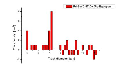
Pd/SWCNT/Pd:D<sub>x</sub> after electrolysis:  $t = 10 \times 3600 \text{ s}$ , 33µm Al and 25µm Cu filtered CR-39 data. Right graph shows 11-16 MeV alpha identification
