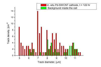
Pd: No statistically significant emissions (besides absorbed natural alpha nuclides) is detected. Pd-SWCNT: Statistically significant emissions of protons and energetic alphas in the one 122 hr run:  $\langle N_p \rangle = (5.24 \pm 1.09) \times 10^{-4} \text{ p/s-cm}^2$ ,  $\langle N_\alpha \rangle = (1.04 \pm 0.15) \times 10^{-3} \alpha/\text{s-cm}^2$
