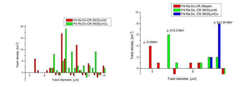
CR-39 track diameter distributions (with the Backgrounds subtracted) for the sum of the Pd/Re: $D_x$ +Pd/SWCNT: $D_x$  runs
