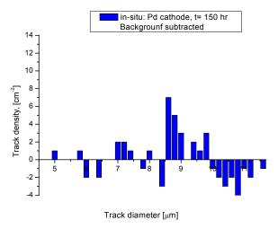
Net SWCNT (D/C = 1.5) contribution in charged particle emissions: the Pd cathode CR-39 result is subtracted from that of the Pd/SWCNT/Pd
