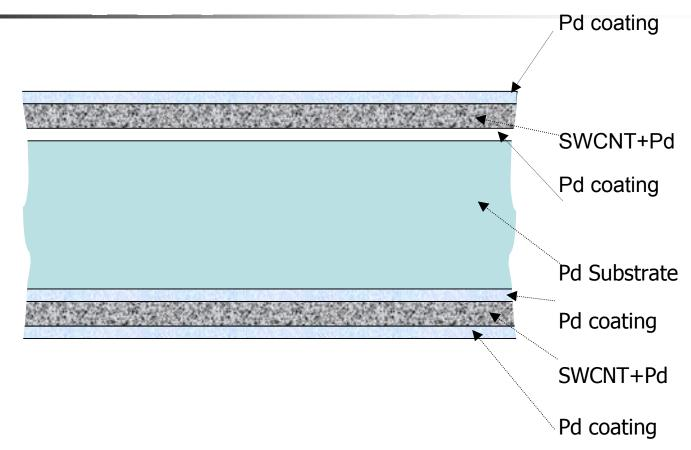
Pd'/SWCNT/Pd'/Pd/Pd'/SWCNT/Pd' composite foil; SWCNT ( $\emptyset = 1.3$  nm) types:
