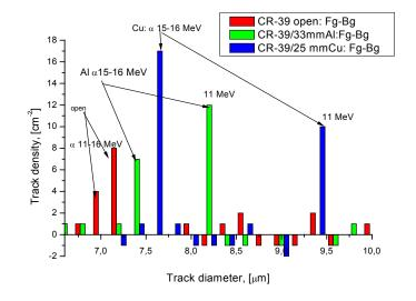
Pd/Re/Pd:D<sub>x</sub> after electrolysis: t = 10x3600 s, open CR-39 data:  $<N_{\alpha}> = (3.43\pm0.76)x10^{-3} \alpha/s-cm^{2}$
