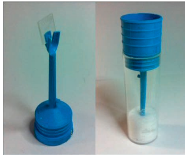
Figure 41 Polystyrene cylinder contains CR-39 detector surrounded by boric acid (images courtesy D. Cirillo).
