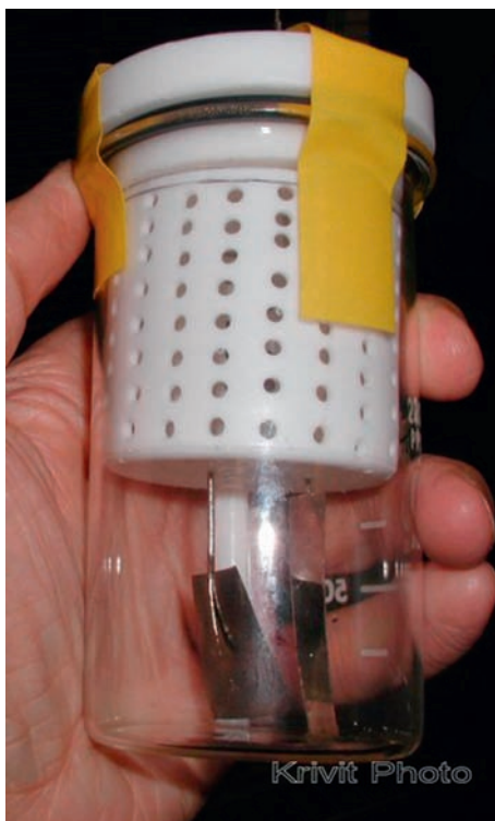
Figure 84 Simple electrolytic cell used by students at Portland State University. During experiment, cathode foil begins to curve and approach anode.
