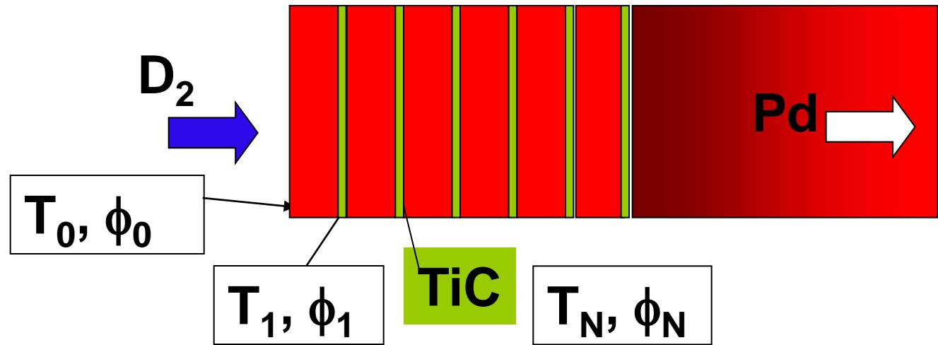
$$T_{0N} = \frac{T_0 * T_N}{T_0 * T_N + (\sqrt{1 - T_0} - \sqrt{1 - T_N})^2 + 4\sqrt{(1 - T_0)(1 - T_N)}(\cos[\frac{\phi_0 + \phi_N}{2}])^2}$$
