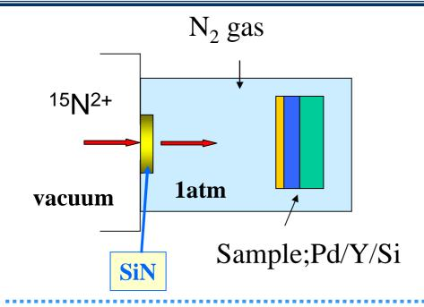
Recently, we made a success to measure hydrogen distribution under normal pressure(~1am).
