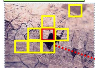
Smaller X-ray beam provides more localized Pr distribution.
