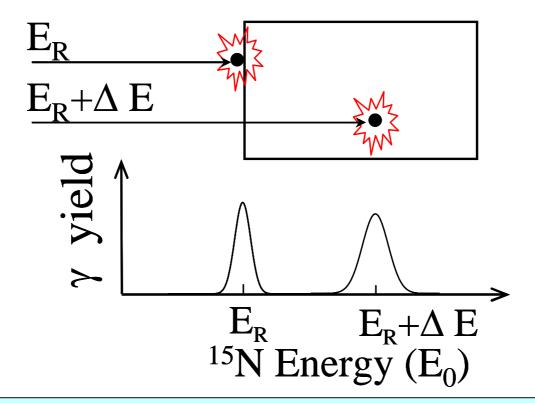
Hydrogen density distribution can be measured by 15N Ion beam
