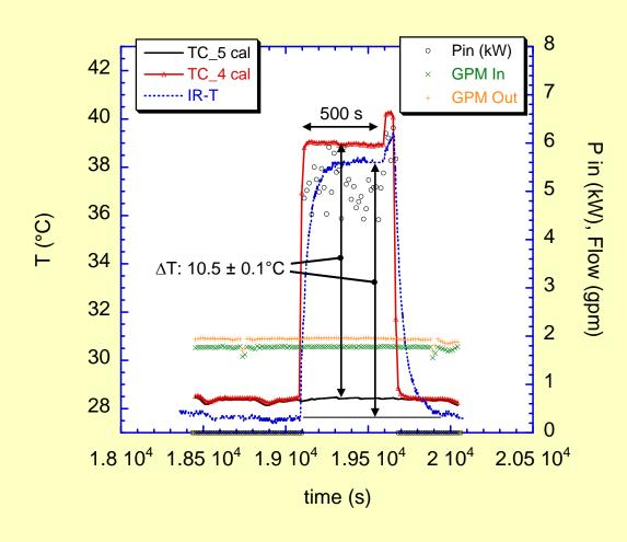
**P**<sub>in</sub> undersampled with power meter, as heater operates in "switching" mode, causing scatter in data.
