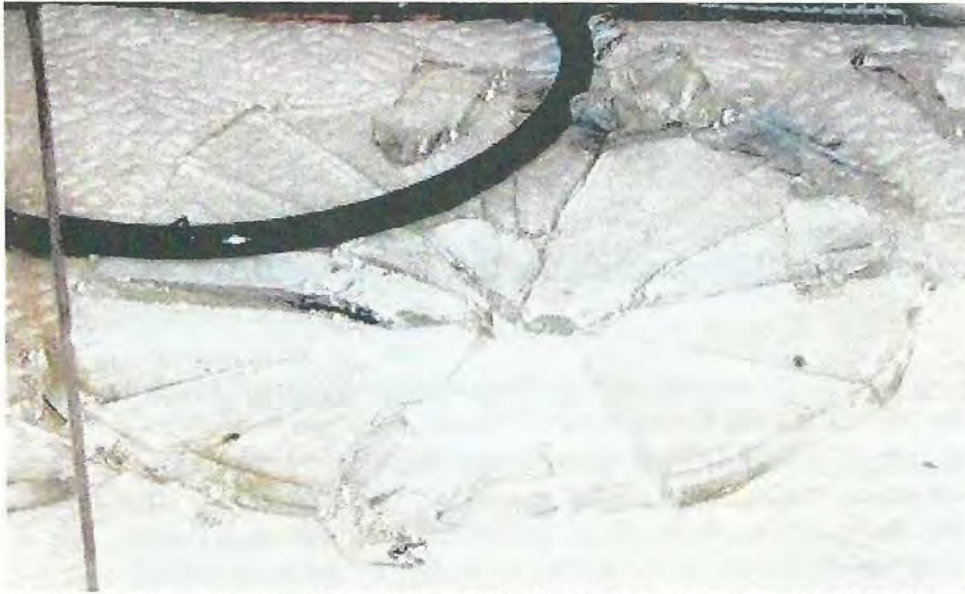
Radial fracture pattern of the bottom of the flask after explosion. Photo by Mizuno.
