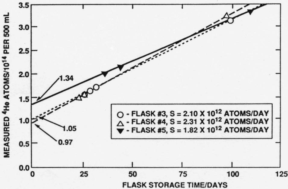
Fig. 2. Experimental rate of atmospheric helium diffusion into three Pyrex flasks filled with D<sub>2</sub> + O<sub>2</sub> from Pd/D<sub>2</sub>O electrolysis. These experiments yielded excess power, helium production, and anomalous radiation, as shown in Table IV.
