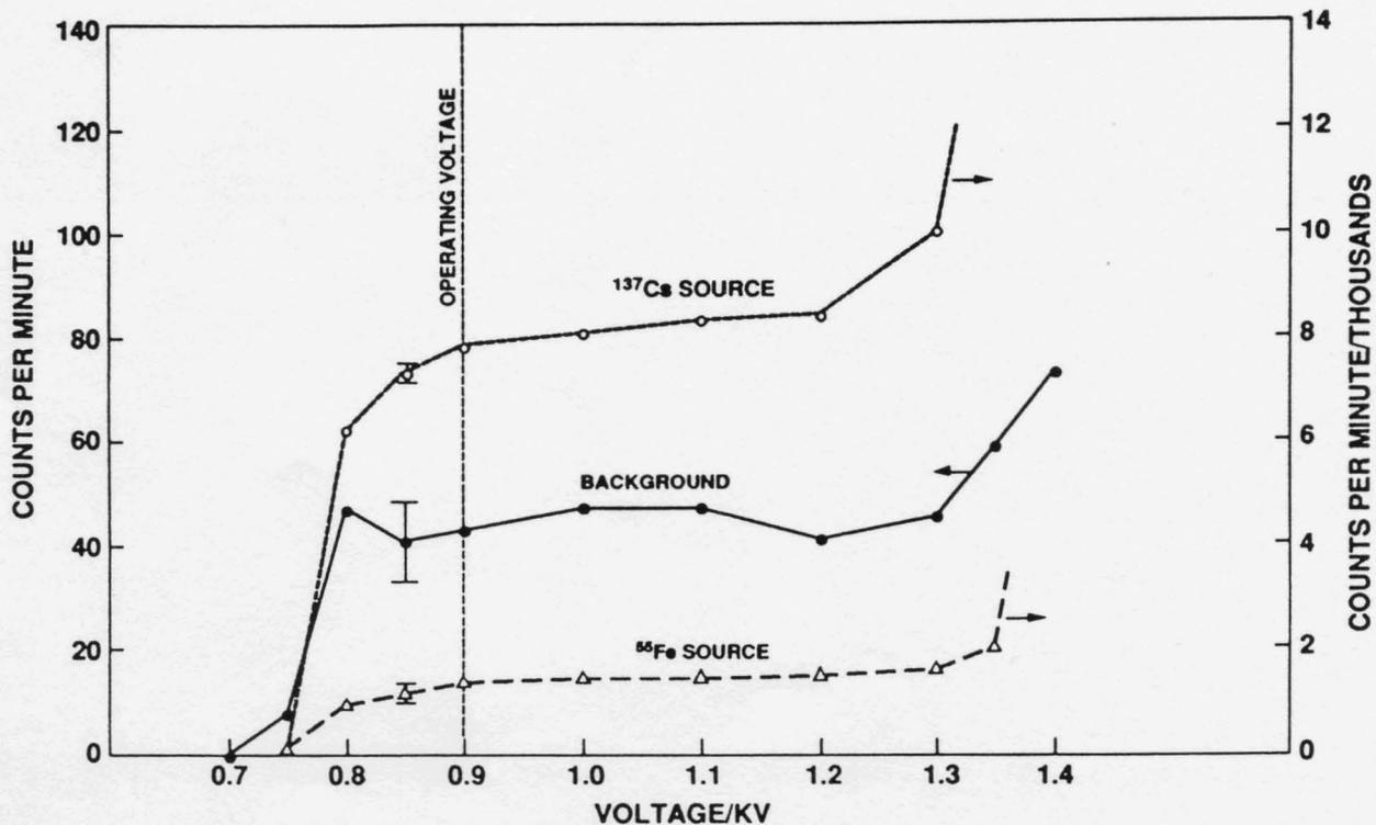
Fig. 5. Plateau determinations for the GM detector with  $^{137}\text{Cs}$  and  $^{55}\text{Fe}$  sources as well as the background counts. Normal behavior is observed. (The error bars represent  $\pm 1\sigma$ .)
