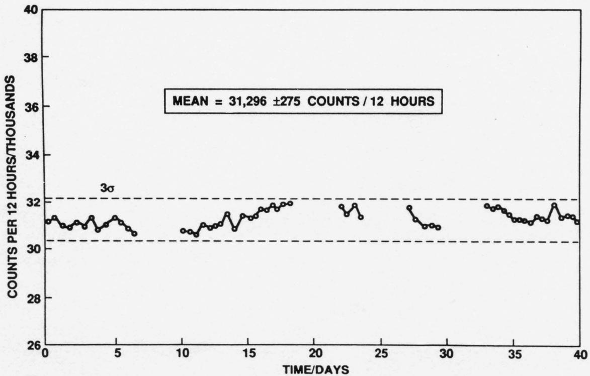
Fig. 4. Radiation counts observed with the GM detector during various experiments that produced no significant excess power. These radiation counts were used to establish the mean background of  $31\,296 \pm 275$  counts per 12 h.
