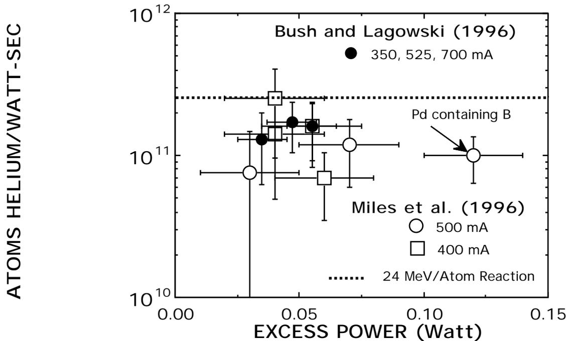
**Figure 12.** The number of atoms of  $^4\text{He}$  collected in a flask while the cell was being electrolyzed using the indicated currents. One sample contained 500 ppm boron and gave the same result as the other samples containing less than 10 ppm boron.
