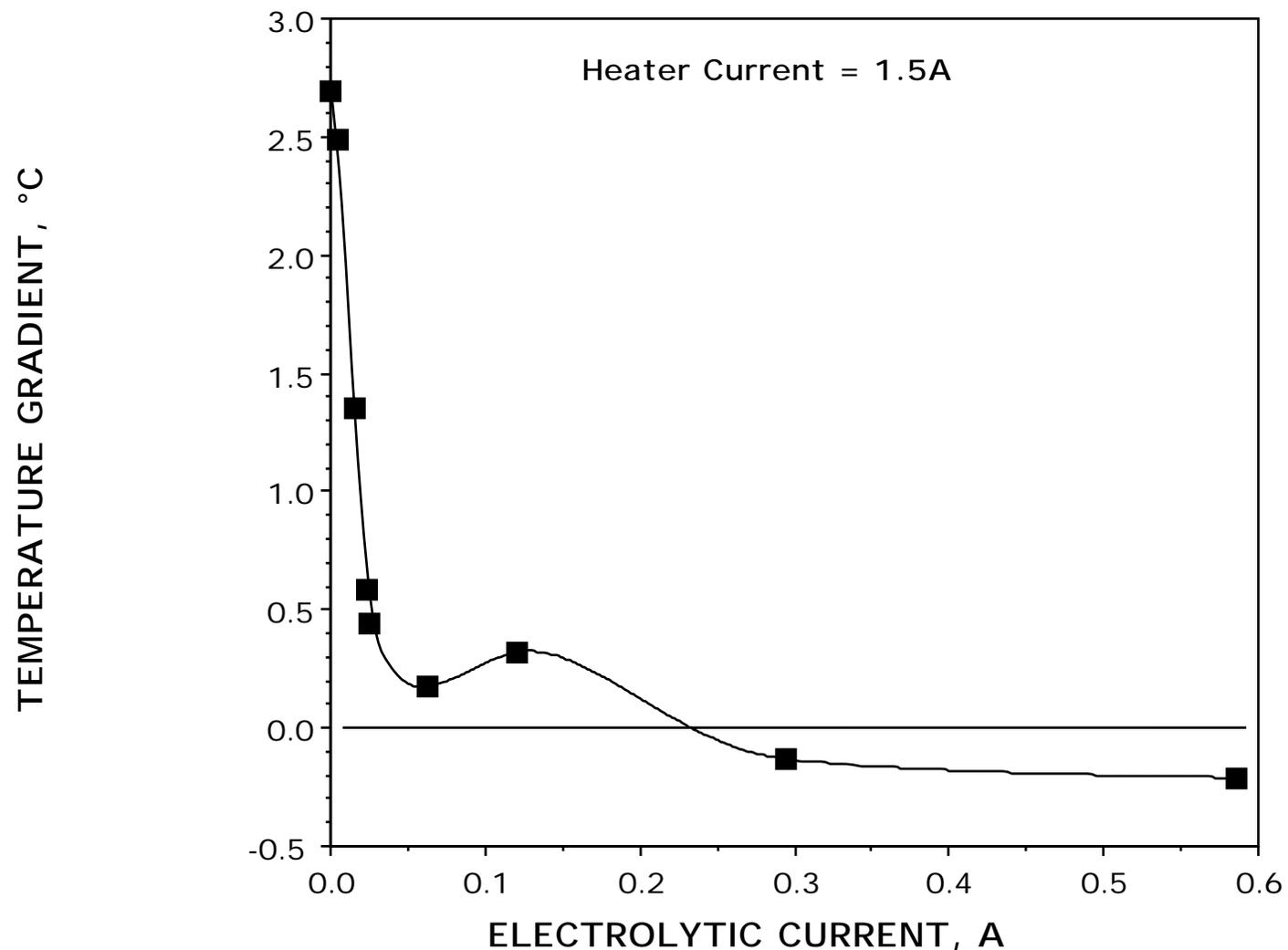
Figure 2. Reduction in gradient as electrolysis current is increased at fixed heater current.
