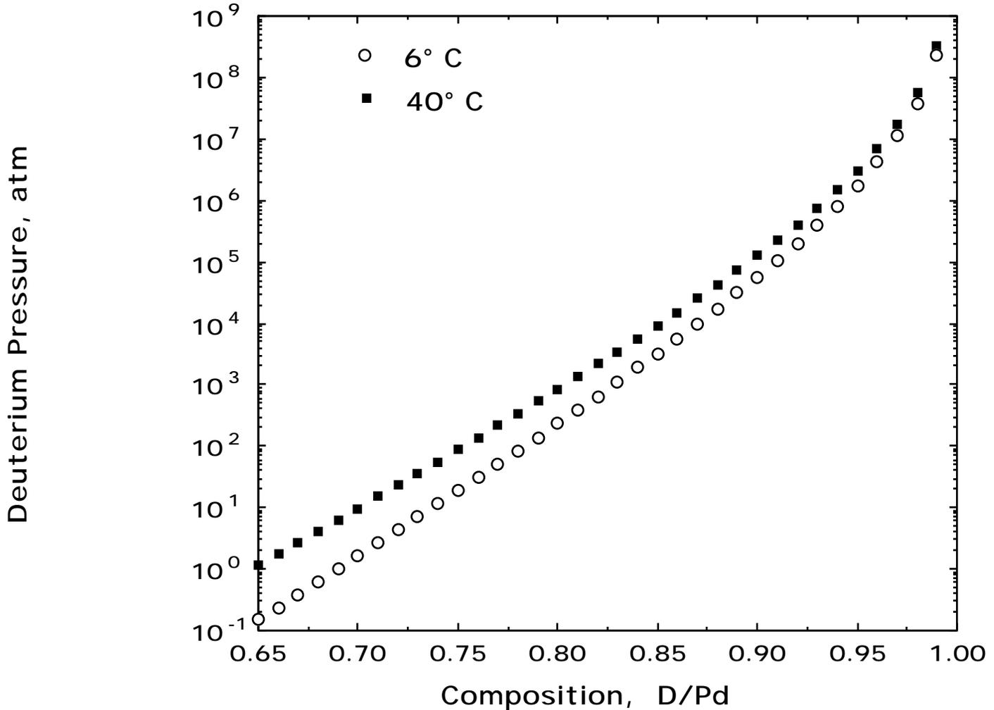
**Figure 13.** Equilibrium pressure of  $D_2$  as a function of composition at two different temperatures.
