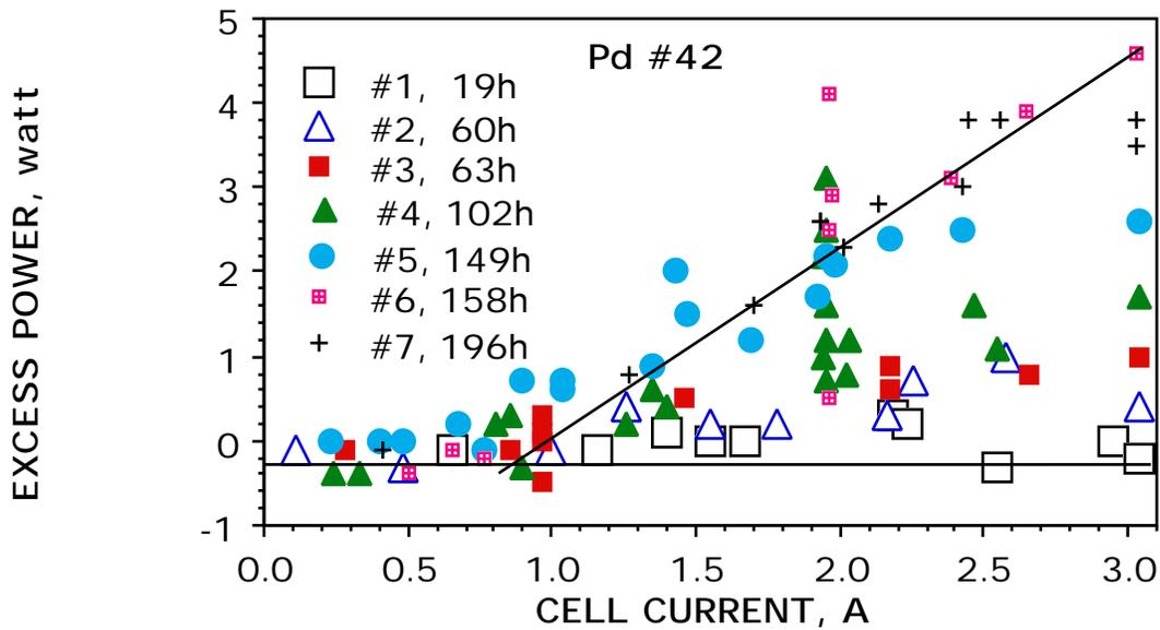
Figure 9. Excess power as a function of applied current shown after various times. The plate had an area of  $4 \text{ cm}^2$ .
