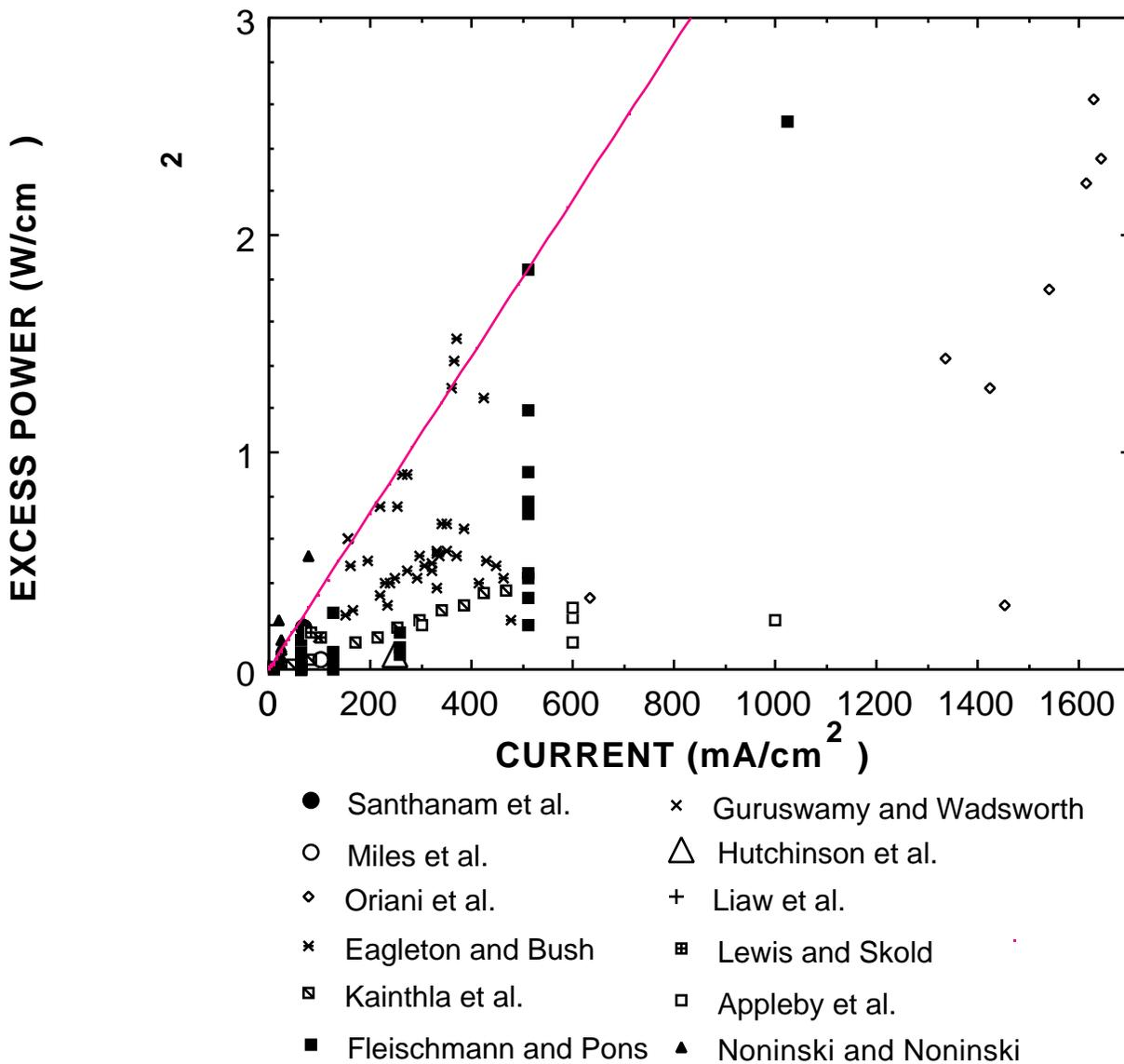
Figure 5. A comparison of power production as a function of applied current density. The line shows the upper limit of all reported values, some of which are off the graph.
