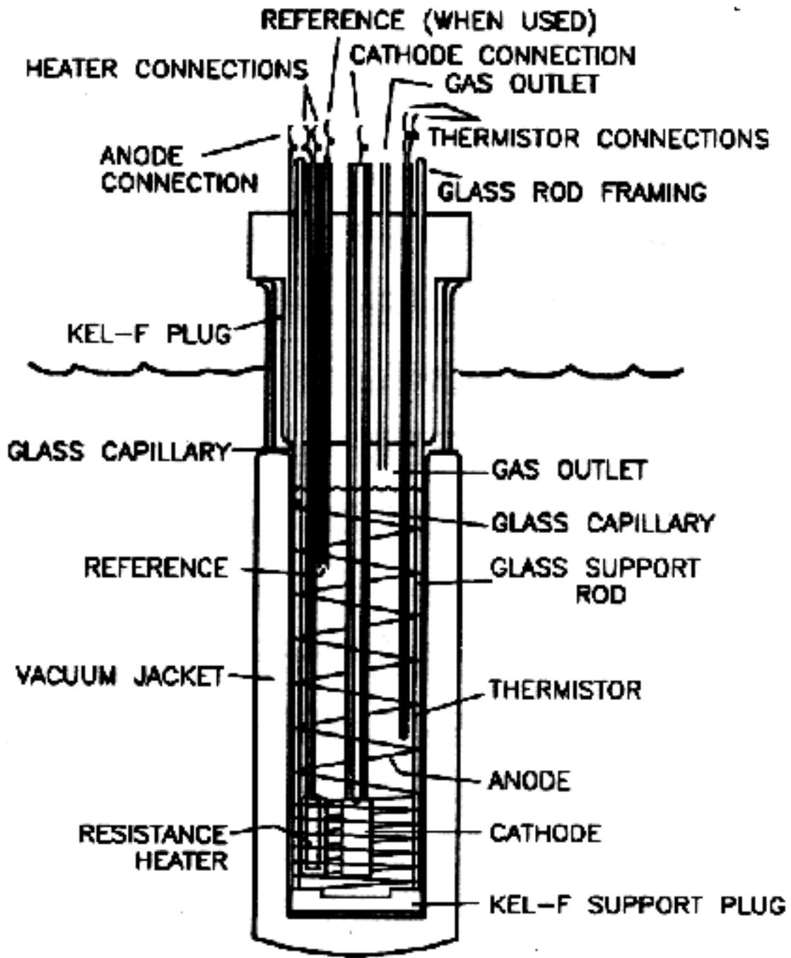
Figure 4. Drawing of P-F calorimeter. The upper section was silvered in later versions.
