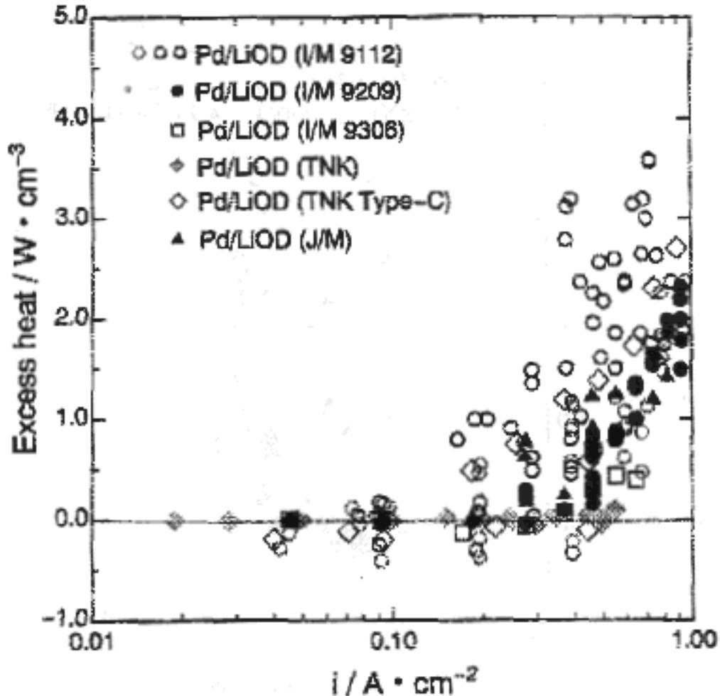
**Figure 11.** Effect of applied current on excess power shown by Hasegawa *et al.*[48]
