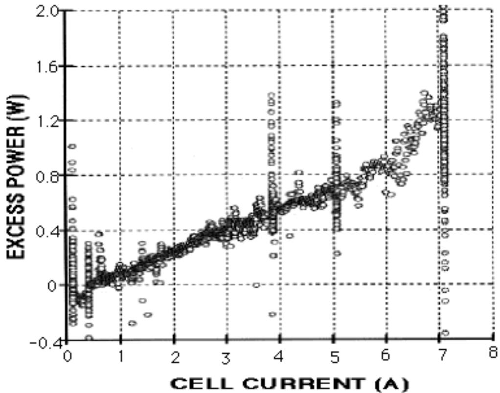
Figure 10 Typical effect of applied current on the production of excess power based on work done at SRI. The critical current varies between samples with a typical value being near  $250 \text{ mA/cm}^2$ .
