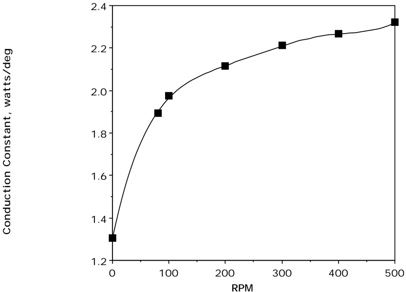
Figure 3. Effect of stirring rate on the effective thermal conductivity of a cell wall. Power is applied electrolytically to a typical cell design. Stirring is done using a Teflon covered magnetic bar located at the bottom of the cell.
