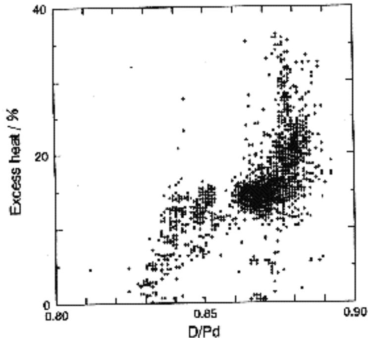
Figure 8. Effect of average bulk composition on production of excess power using palladium wire.
