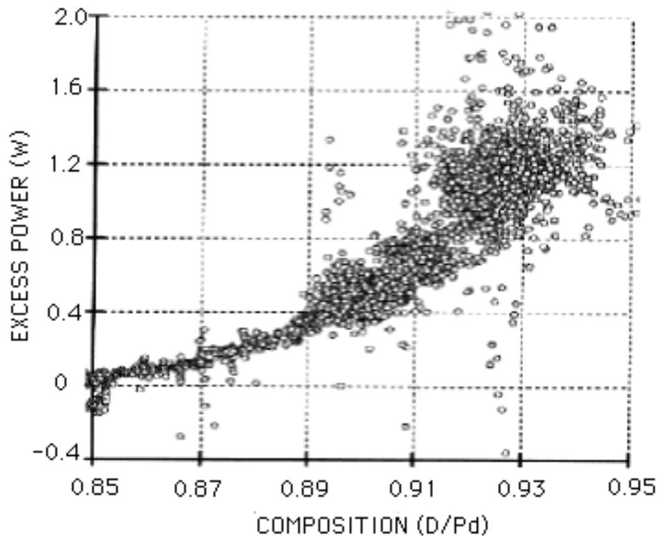
**Figure 6.** Typical effect of average bulk composition of a wire on the production of excess energy. Data was obtained at SRI using a flow calorimeter. Composition is based on changes in resistivity.
