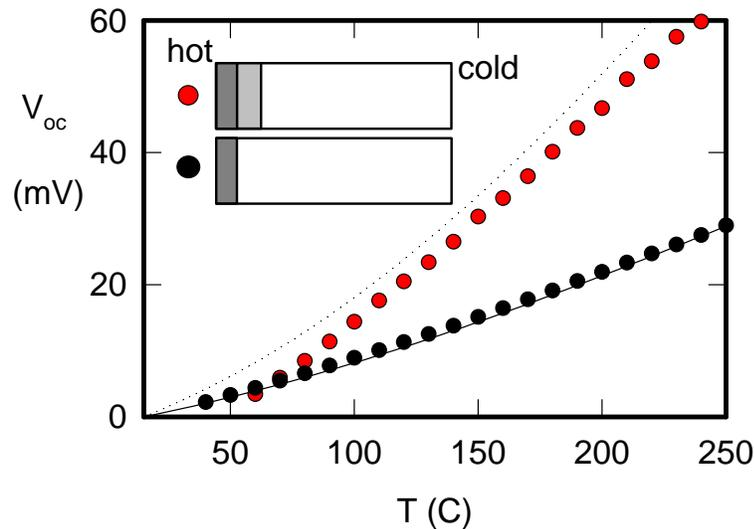
**Figure 1.2** Open-circuit voltage as a function of current for an InSb thermal diode with a poor emitter (black solid circles); thermoelectric model open-circuit voltage (solid line); open-circuit voltage of a thermal diode with a good emitter (red solid circles); model open-circuit voltage calculated from the current injection model (dotted line). Current injection from the emitter has increased the open-circuit voltage by a factor of 2.2 over the thermoelectric result.
