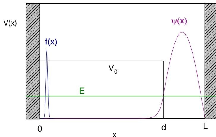
**Figure 3.2** Schematic of 1-D analog model. The molecular potential is modeled by a square well with zero potential between  $d$  and  $L$ , and a constant potential below  $d$ . The unperturbed ground state (analog for the molecular ground state) is illustrated as  $\psi(x)$ . Dissociation of helium leads to two deuterons with a tiny separation. This is accounted for in the function  $f(x)$ .
