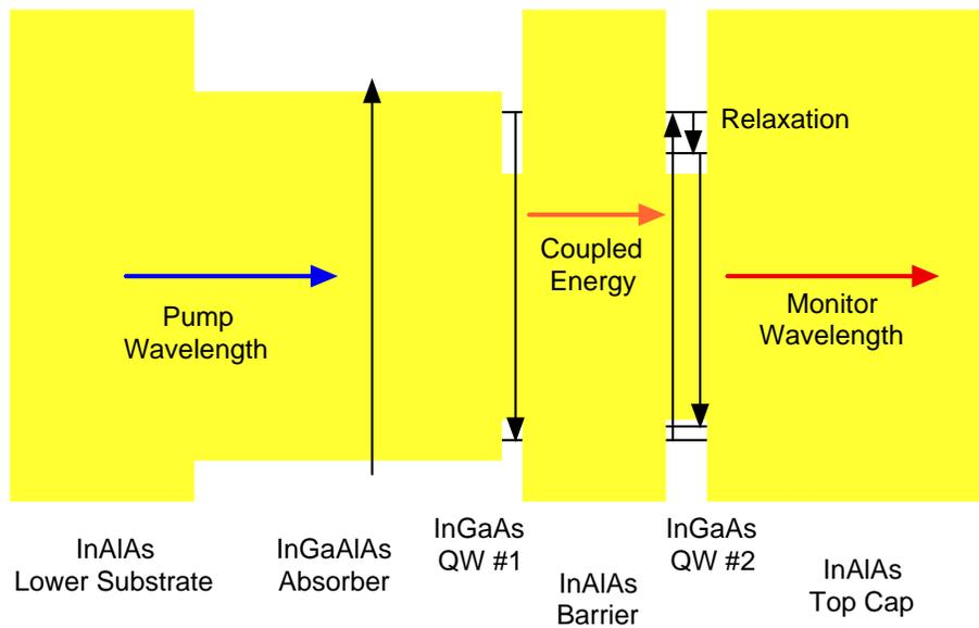
**Figure 2.3.** QW test structure to probe proximity and resonance coupling.
