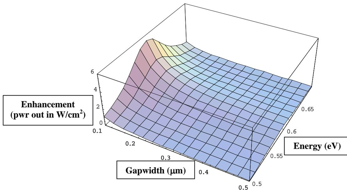
**Figure 2.2** An example of proximity enhancement for resonant states at 0.6 eV. Effects of gapwidth and line broadening are displayed.
