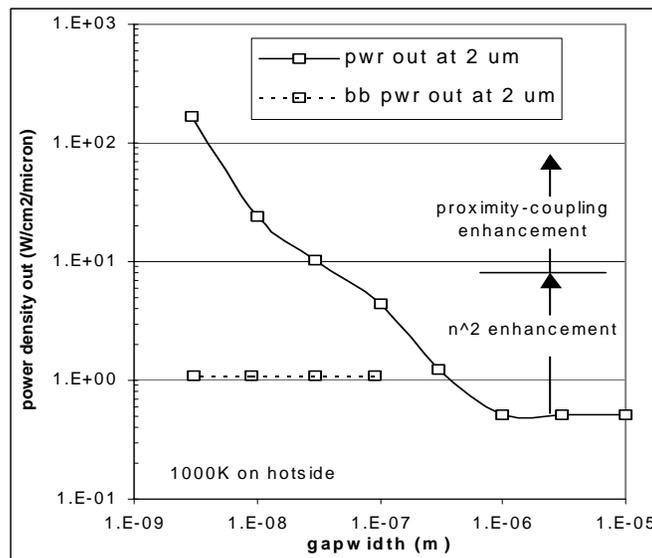
**Figure 2.1.** Electromagnetic theory enhancement model results. Output power density for 2  $\mu\text{m}$  light from a silicon emitter into an InGaAs TPV detector.
