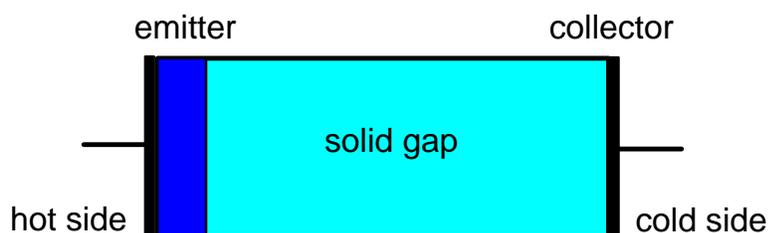
**Figure 1.1** Basic thermal diode structure. Second-order thermionic current injection from the heavily doped emitter diffuses across the solid gap region to the collector. The solid gap region is a near-intrinsic thermoelectric semiconductor, which contributes a thermoelectric current in addition to the injected current.
