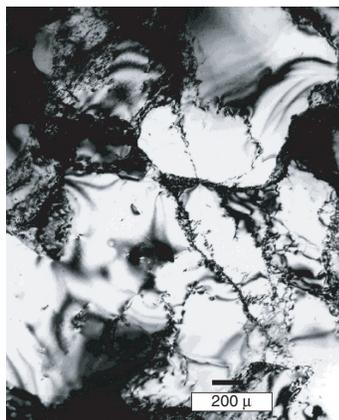
Figure 7. Palladium annealed at 1100°C for 5 h.
