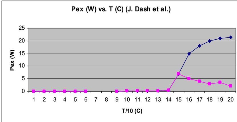
Fig. 4. Temperature dependence of the excess energy  $P_{ex}$  (W) from three experimental data sets obtained between June 20, 2006 and January 18, 2007. The high temperature region after bifurcation is an estimate, as explained in the text.
