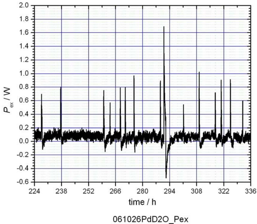
Fig. 2. Excess power bursts during a 112 hour period of an experiment which lasted 14 days.
