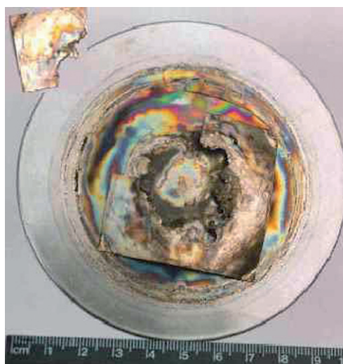
Fig. 8 Two pieces of metal: A 50 × 50 × 0.01 mm Pd foil in front of a 40 mm thick 10 cm stainless steel disk. The pieces were used together by Stringham during a 20-hour acoustic cavitation experiment. The only power applied to the experiment was applied acoustically from a 500 Watt Misonix’s 5 cm Ti acoustic horn. The colored pattern on the stainless steel disk is caused by the migration of Pd atoms to the disk. The thin layer of Pd or palladium oxide deposits on the stainless steel disk and the condition of the melted Pd foil indicate very high transient and local temperatures sufficient to vaporize Pd. This experiment was performed around 1994-1995. 11 Photo: R. Stringham.
