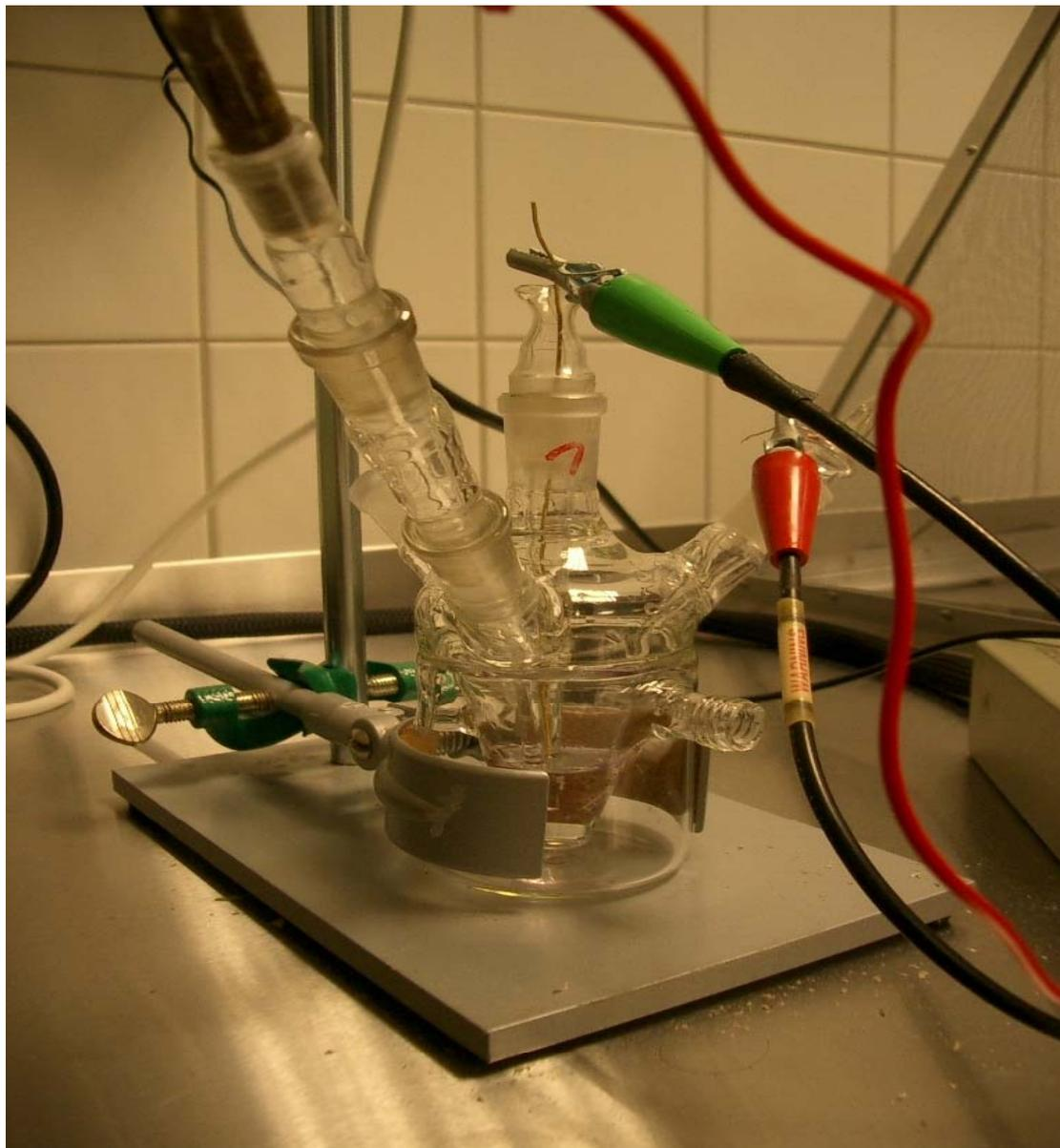
Fig 3: Scheme of the electrolysis cell (1) Teflon caps; (2) glass rod; (3) Pd rod; (4) glass beaker; (5) Pt Coil. (Pg 191, Chun-Ching Chien, Dalibor Hodko, Zoran Minevski, and John O'M. Bockris, J. Electroanal. Chem. 338 (1992) 189-212)
