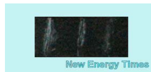
CR-39 detector after exposure to LENR experiment. Detector shows—to the naked eye—the clearly marked pattern of the three cathode wires used in the experiment. Photograph is actual size, zero magnification. Photo: Steven Krivit
