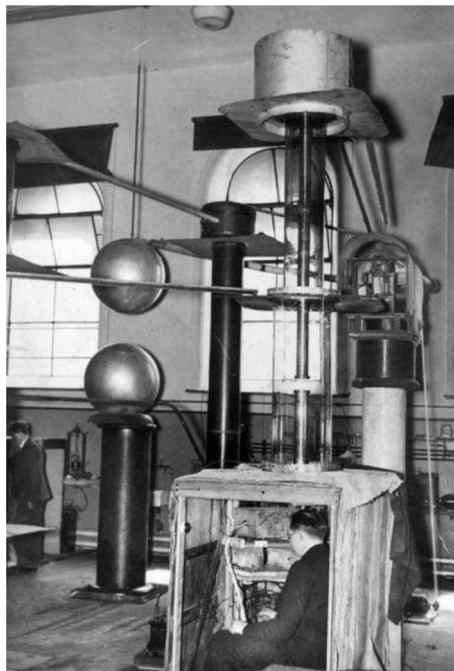
Figure 8. The apparatus with which Cockcroft and Walton artificially disintegrated lithium nuclei (Cockcroft and Walton 1932). Walton is sitting inside the little tent, observing the decay products on a luminescent screen. Cockcroft is on the left.
