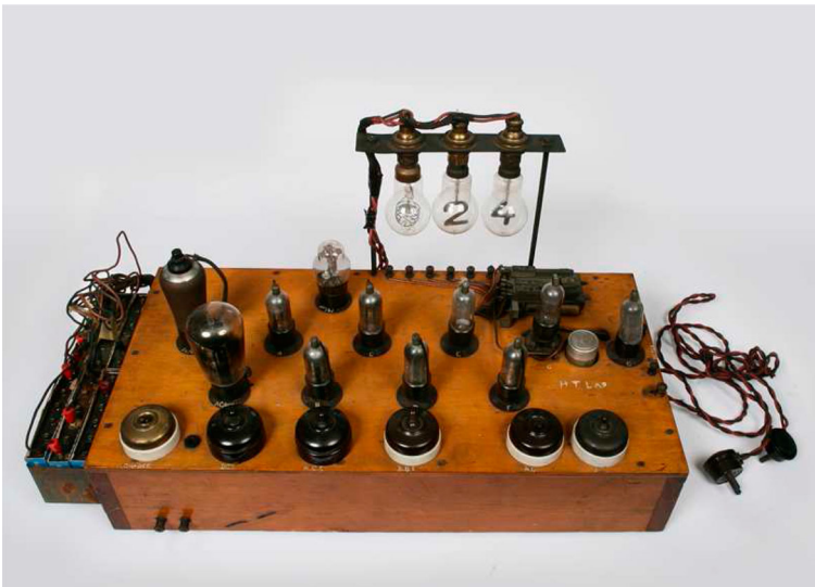
Figure 5. A ‘next vintage’ version of the Wynn-Williams’ scale of two counters. In the 1980s, he tried to find the original, but it was long gone. This second generation counter survived (Wynn-Williams 1984).
